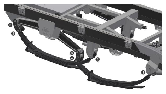
We recommend a high-quality grease with a molybdenum-disulphide lithium base for chassis lubrication.
