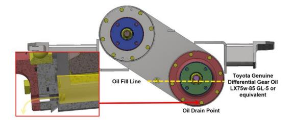
**DRAINING PROCEDURE** - Remove the bolt from the bottom of the chain case (one of the 8 bolts holding the mid output bearing case) to drain, and refit when thoroughly drained.
