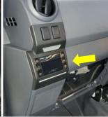
**23.** Connect the LHS display panel and RHS LED light panel connectors. Carefully clip the left and right-side panels into the dash.
