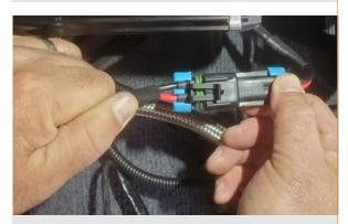
**39.** Connect power connector to compressor.
