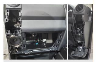
**10.** Dash/center console area is now prepped for display panel harness installation.
