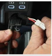
**7.** Connect the supplied T harness to the factory 12V connector and route the complete harness through the socket hole. Pull it out from the glovebox opening while leaving the white male connector of the T harness hanging outside.
