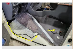
**33.** Route the battery harness along the door sill channel and across to the carpet cut. Pull the harness through the cut.
