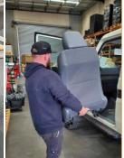
**2.** Using a 14mm socket remove 4x seat mounting bolts. Rear seat mounting bolts are behind plastic covers. Carefully remove the front passenger seat from vehicle – take extra care not scratch plastic or painted surfaces.
