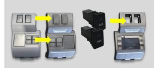
19. Remove and transfer existing factory switches to driver side panel. Install the provided AUX switches into the passenger side panel. Note: to adapt driver side switch insert to suit pre 20MY vehicles, see supplement page 14 of this guide.
