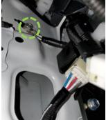
**29.** Route the ground wire up and into the passenger side footwell. Use a 10mm socket or spanner to remove the factory bolt. Mount the ground wire eyelet, return the factory bolt and tighten till secure.
