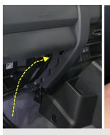
**4.** Reach through glove box opening and locate the back side of the 12V socket. Apply gentle pressure to the back of the socket as you release the interior retention clip. The socket will unclick and slide out.
