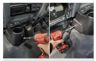
8. Use a 10mm socket to remove the two bolts securing the center console cup holder. Note: For steps on installing IGN harness in 24MY+ automatic vehicles, see supplement pages 12-13 of this guide.
