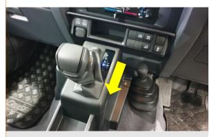
**1.** Turn key to the ON position, press the brake pedal and shift the gear lever to D.
