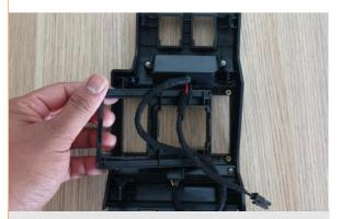
**3.** Remove the factory fitted switch panel.
