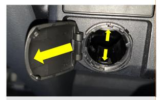
**6.** Locate the two locking clips inside the socket lid unit. Gently lift each one up while pulling the complete unit with light pressure. The unit will unclick and slide out.
