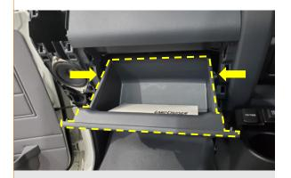
**5.** Remove glovebox by compressing the sides until glovebox hinges disengage. Glovebox can now be unclipped from the bottom and removed.
