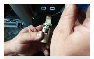
**5.** Use pin removal tool to release the connector lock and unplug socket from factory 12V harness.
