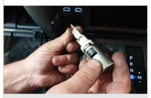
**9.** Connect the 12V power socket cylinder unit to the male white connector.
