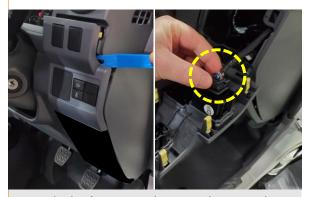
**7.** With the lower panel removed, use a plastic tool to remove the upper panel. Carefully disconnect connector from back side of panel.
