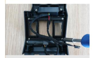
**5.** Reinstall the four Phillips screws.
