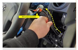
**13.** Pull passenger side panel connector through cavity.
