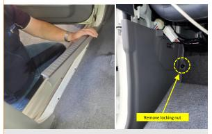
**3.** Use a Phillips screwdriver to remove screws securing the door sill protector and a plastic tool to remove the protector. Remove the plastic nut securing the footwell kick plate.
