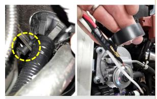
**31.** Locate the passenger side firewall grommet and use scissors or a sharp blade to remove the tip from the available nipple. Attach the battery harness to a wire puller and feed through the grommet nipple.
