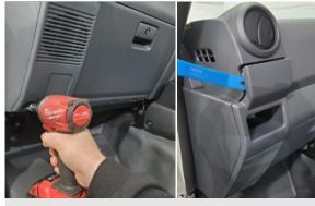
**4.** Using a 10mm socket remove the bolt securing the lower plastic trim panel. Lower panel must be removed to allow removal of upper panel. Use a plastic tool to remove upper panel.
