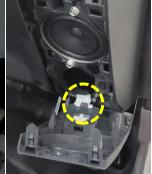
**6.** Use a 10mm socket to remove the bolt securing lower plastic panel. Use a plastic tool to remove the panel. **DO NOT** disconnect bonnet release cable.
