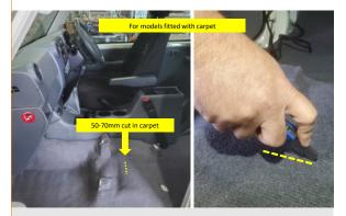
**24.** For Vehicles with carpeted floor only. To route the main display connector harness, and BATT, IGN and GND harnesses you will need to use a sharp blade and cut a 50-70mm hole in the carpet below the front passenger seat.
