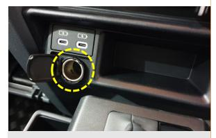
**2.** IGN T harness will be routed through the 12V socket and across to the glovebox area. Open the 12V socket cover to begin socket removal process.
