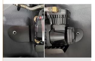
**41.** Ensure compressor mounting bracket bolt holes are correctly aligned with factory seat bolt holes before returning passenger seat.
