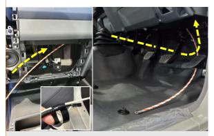
**12.** Attach RHS panel connector to wire puller and pull through center console and up into the RHS speaker cavity. Be careful to avoid pedal mechanisms and steering components.
