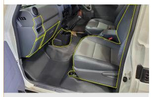
**1.** Prepare interior for installation by completely removing passenger side front seat, glovebox, passenger and driver side dash trim pieces and cup holder/USB console. See steps 2-10 for detail.
