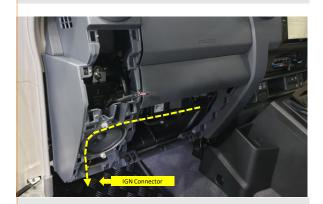
**11.** IGN harness connector should be routed behind the glovebox towards front passenger footwell area.
