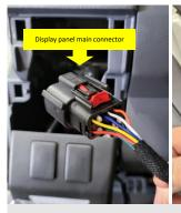
**21.** Route the LHS Display panel harness and connector into LHS cavity and down to the front passenger footwell area.
