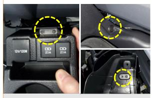
**9.** Remove 2x Phillips screws at backside of console and plastic clip. Console can now be removed from mounting bracket. Remove 2x Phillips screws from bottom of console to access 12v connectors.
