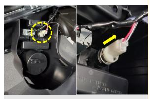
15. Remove the factory connector from the back of the vehicle 12V accessory socket. Note: For steps on installing IGN harness in 24MY+ automatic vehicles, see supplement pages 12-13 of this guide.
