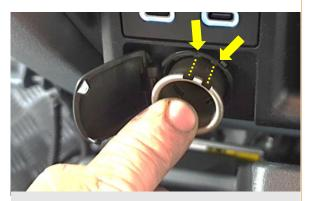
**10.** Insert the socket in its place and click lock it. Make sure the cutouts on the edges of the cylinder are aligned to the plastic tabs on the lid unit.
