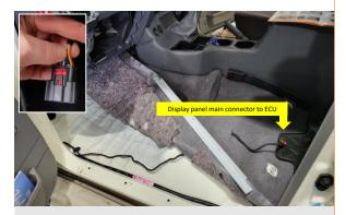
**25.** Route the main display connector along the door sill channel and across to the hole in the carpet/vinyl. Pull the connector through the hole and leave ready for connection to compressor ECU.
