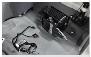
**37.** Carefully place the compressor unit into the installation area.
