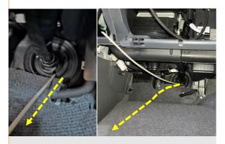
**32.** The wire puller will exit in the passenger side footwell, pull the battery harness through to the vehicle interior.
