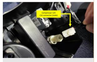
**17.** Connect the control panel IGN connector to the vehicle 12V accessory socket.
