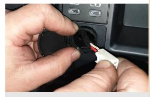
**8.** Reinstall the power socket lid unit back into its place and click lock it.
