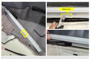
**34.** Use a sharp knife to cut a portion of the under carpet/vinyl plastic edge material as per picture. This will create a channel for the compressor harnesses to pass through.
