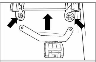
**2.** Using a 14mm socket remove the two front passenger seat mounting bolts. Lift the front of the seat slightly to allow the mounting bracket to slide underneath.
