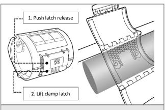
**4.** Open the quick release clamp and mount your chosen 80mm diameter extinguisher bottle as shown. Close the clamp and secure the clamp latch.
