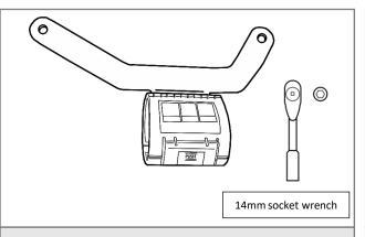
**1.** Your Quick Release Extinguisher Clamp is designed to be installed at the base of the front passenger seat using the existing seat mounting bolts.
