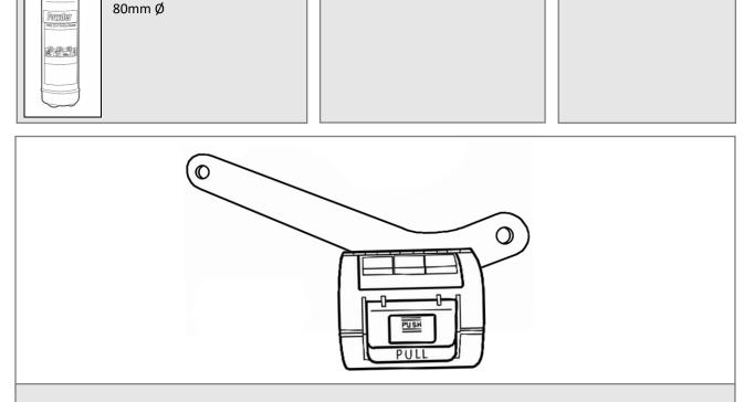
**1.** Your Quick Release Extinguisher Clamp is designed to be installed at the base of the front passenger seat using the existing seat mounting bolts.
