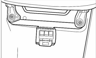
**3.** Using a T45 Torx socket or Key reinstall the two front passenger seat mounting bolts. Be sure to tighten the bolts securely. You can now mount Fire Extinguisher bottle into your Quick Release Clamp.
