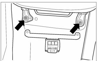
**2.** Using a T45 Torx socket or Key remove the two front passenger seat mounting bolts. Lift the front of the seat slightly to allow the mounting bracket to slide underneath.
