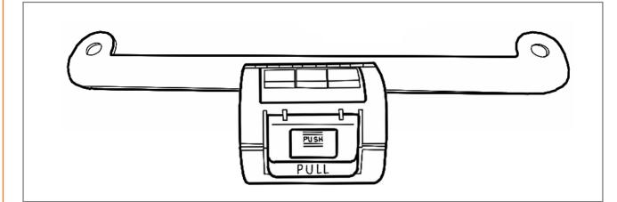
**1.** Your Quick Release Extinguisher Clamp is designed to be installed at the base of the front passenger seat using the existing seat mounting bolts.
