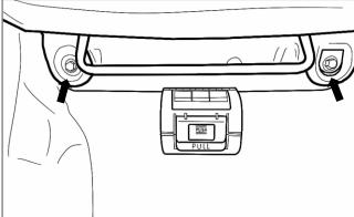
**3.** Using a 14mm socket reinstall the two front passenger seat mounting bolts. Be sure to tighten the bolts securely. You can now mount Fire Extinguisher bottle into your Quick Release Clamp.
