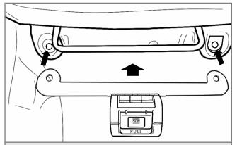
**2.** Using a 14mm socket remove the two front passenger seat mounting bolts. Lift the front of the seat slightly to allow the mounting bracket to slide underneath.
