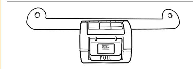
**1.** Your Quick Release Extinguisher Clamp is designed to be installed at the base of the front passenger seat using the existing seat mounting bolts.
