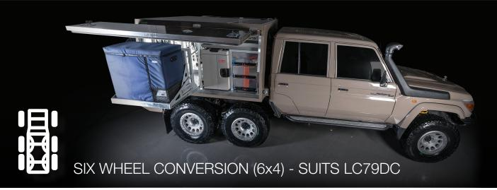
Convert the Toyota LC79 dual cab 4x4 to a Multidrive Technology 6x4 and benefit from massive load carrying capacity. Enjoy improved and predictable handling characteristics whilst remaining safe and legal. Whatever the conditions – heavy loads, towing, or rough offroad tracks – Multidrive Technology drives your payload further!
